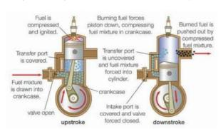
Before the 2-stroke cycle can begin, the fuel mixture needs to be introduced, which requires an initial upward movement of the piston, initiated by either a starter motor or kick-start. This upward movement creates a slight suction in the crankcase and uncovers the intake port, so that fuel mixture is drawn from the carburettor into the crankcase. After reaching top-dead-centre, the piston begins its downward stroke (the beginning of the 2-stroke cycle),
