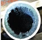
This is what I found deeper down, when the Header was sectioned. It may look like a rubber sleeve inside the pipe but it's a really hard, baked on oil and carbon mix.
